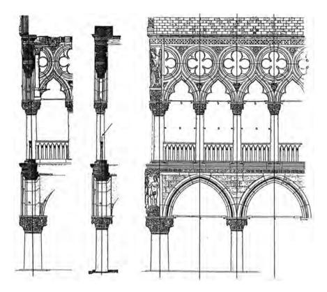
**Figure 3.** Venice, Palazzo Ducale, (left) section through south facade, begun 1341, taken through the central balcony of 1404; (right) detail of elevation. From Manfred Schuller, 'Il Palazzo Ducale di Venezia: Le facciate medioevali', in Francesco Valcanover and Wolfgang Wolters (eds.), *L'architettura gotica veneziana* (Venice, Istituto Veneto di Scienze, Lettere ed Arti, 2000), p. 430, fig. 92.
